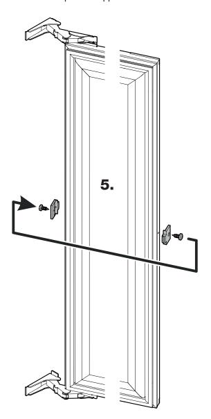
**6.** Unscrew hinges and covers and re-fit on the opposite side at diagonals to the original position.
