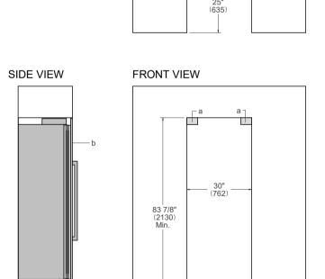
(a) Area to be left clear for the anti-tipping brackets – 3"1/2x5" (82x127mm)
